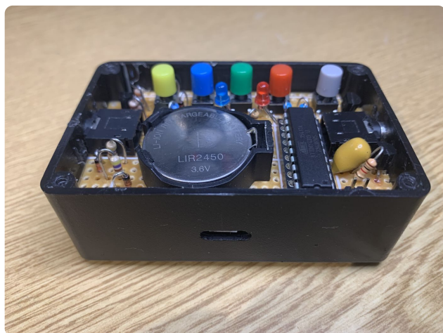
Figure 1: Example layout of the complete version: perforated board with the ATtiny4313 microcontroller and the LIR2450 Li-ion battery. The TP4056 charging electronics are located underneath the board.
