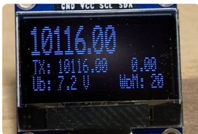
Figure 4: 0.96" SSD1306 I 2 C OLED display, 128 × 64 (connections GND, VCC, SCL, SDA).
