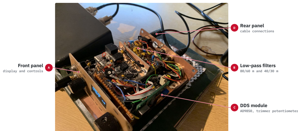
Figure 12: The author's ZB-4 with the enclosure open. Callout positions are approximate.
