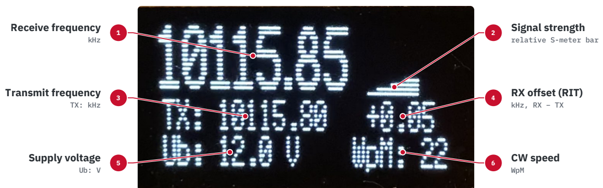
Figure 7: Main screen on 30 m. In this example, the receiver is tuned 0.05 kHz (50 Hz) above the transmit frequency.
