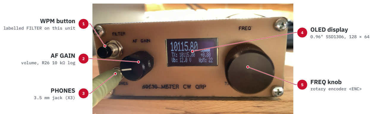
Figure 6: Front panel of the author's build. The panel legend “40/30 METER CW QRP” is struck through on this unit; the ZB-4 covers 80/60/40/30 m.
